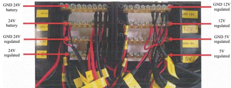
**Figure 7.3:** *Odi* power supplies, exhibiting the 5V, 12V and 24V voltage lines.
