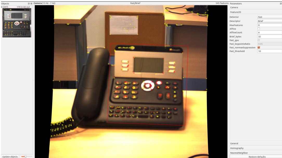
Figure 6.5: How detections are shown on the *find\_object\_2d*'s GUI.
