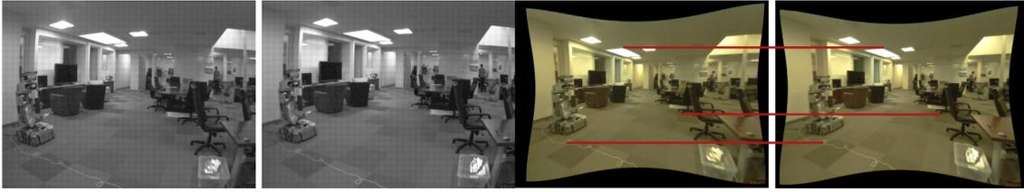
**Figure 4.7:** Pair of raw images (left) and pair of rectified images (right) with two epipolar lines, from [http://wiki.ros.org/stereo\\_image\\_proc](http://wiki.ros.org/stereo_image_proc).
