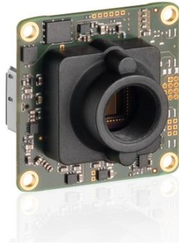
**Figure 4.7:** *Front side of the  $\mu$ eye camera UI-3241LE-C-HQ.*
