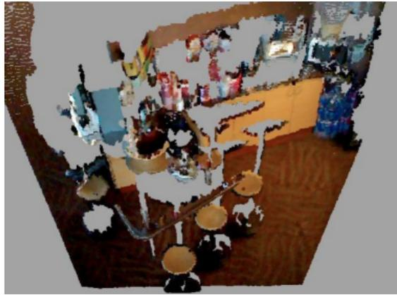
**Figure 4.17:** Example of an RGB-D point cloud.
