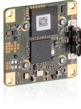
**Figure 4.8:** *Back side of the  $\mu$ eye camera UI-3241LE-C-HQ.*
