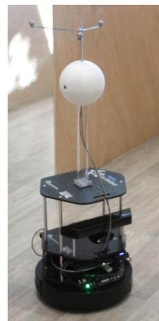
**Figure 6.5:** The binaural spherical head and its mounting on the *turtlebot*
