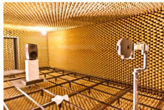
Fig. 2.2: Setup of the measurement in the anechoic chamber of FH Köln.
