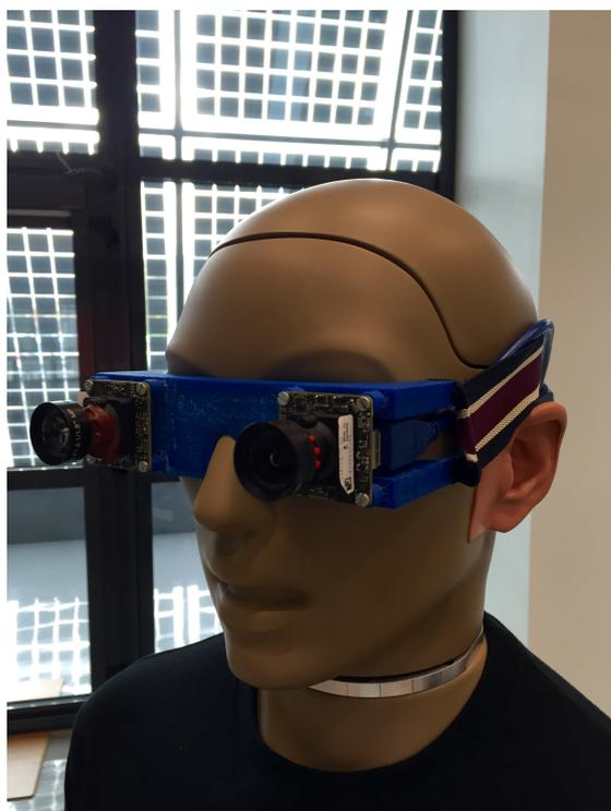
Fig. 6.3: KEMAR head with mounted stereo cameras.
