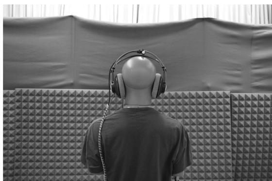
Fig. 2.6: KEMAR wearing AKG K601 headphones in front of the loudspeaker array hidden by a acoustically transparent curtain.
