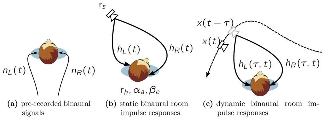
**Figure 3.1:** Techniques for binaural synthesis applied in Two!EARS. Left/right binaural signals are denoted by  $n_{\{L,R\}}(t)$ , BRIRs by  $h_{\{L,R\}}(t)$ , time-variant BRIRs by  $h_{\{L,R\}}(\tau, t)$ . The source signal is denoted by  $x(t)$ , the source and receiver position by  $r_s$  and  $r_h$ , respectively.
