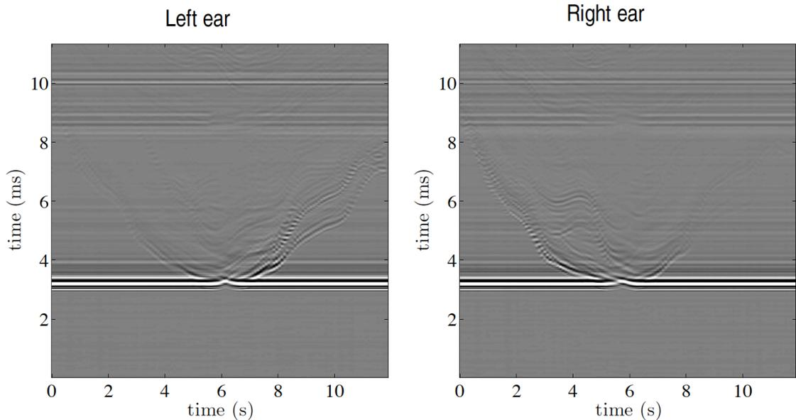
**Figure 3.2:** Dynamic BRIRs captured in a typical office room using a static loudspeaker and HATS position. The horizontal axis denotes the time  $t$  at which a BRIR has been captured. The vertical axis shows the time axis  $\tau$  of the BRIR. A vertical slice represents a BRIR at a given time. A moving scatterer is obstructing the direct path between loudspeaker and HATS at  $t \approx 6$  s.
