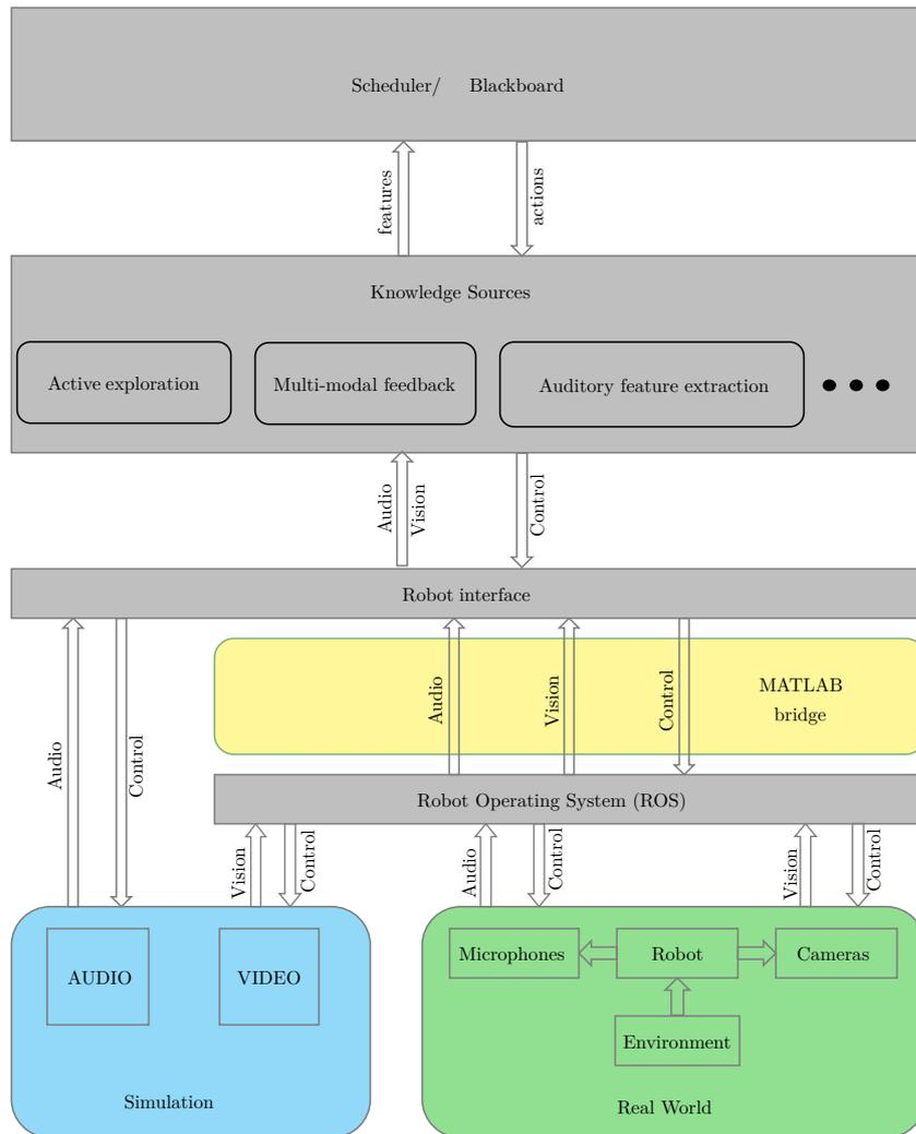
**Figure 2.1:** Architecture of audio-visual simulation framework.
