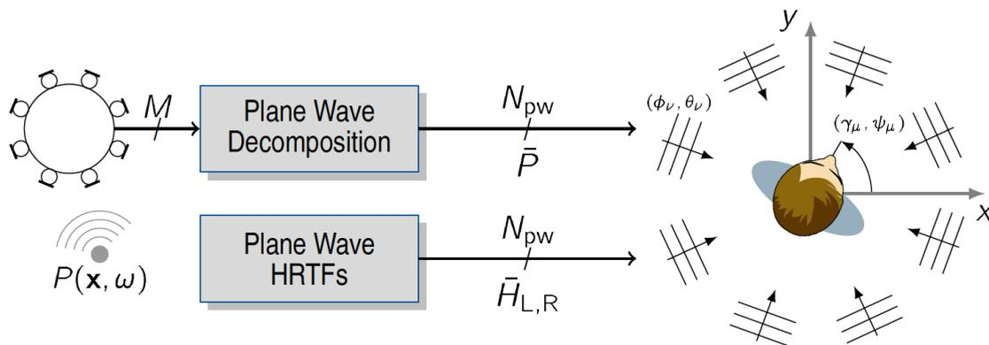
**Figure 3.3:** Data-based binaural synthesis including small scale translatory movements of the listener. The number of microphones is denoted by  $M$ , the number of plane waves by  $N_{pw}$ , the coefficients of the plane wave decomposition by  $\bar{P}$ , the left/right far-field HRTFs by  $\bar{H}_{L,R}$ . The incidence angles of the plane waves is denoted by  $(\phi_\nu, \theta_\nu)$ , the look directions of the listener by  $(\gamma_\mu, \psi_\mu)$ .
