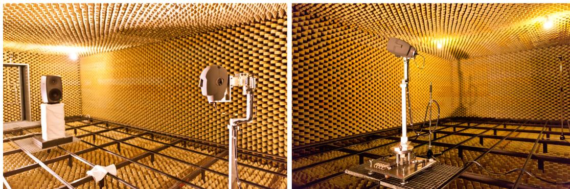
Three-dimensional HRIR datasets were measured with the Neumann KU100 dummy head. An active 3-way loudspeaker (Genelec 8260A) was used as a sound source with a constant distance of approximately 3.25m. Different apparent source positions were realized by rotating the dummy head around two axis using the VariSpear measurement system [26]. The impulse responses were captured for different sampling configurations of the source's position:
