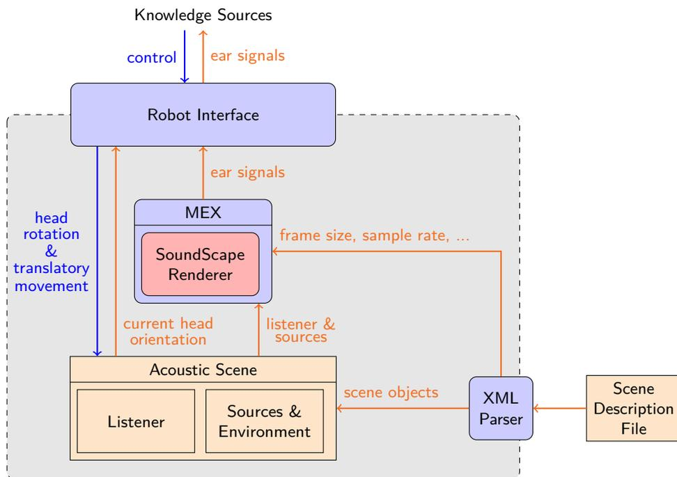
**Figure 3.4:** Software architecture of the binaural simulator
